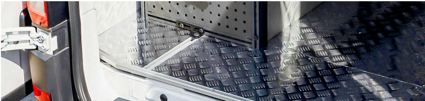
Lightweight and robust van floor with anti-slip aluminium tread plate
